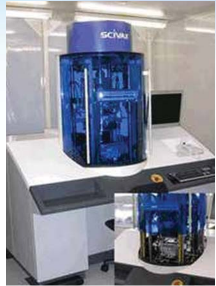
Photo of nano-imprinting instrument SCIVAX VX produced by SCIVAX Co.,Ltd.
